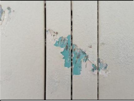
Damage from the first pallet test
